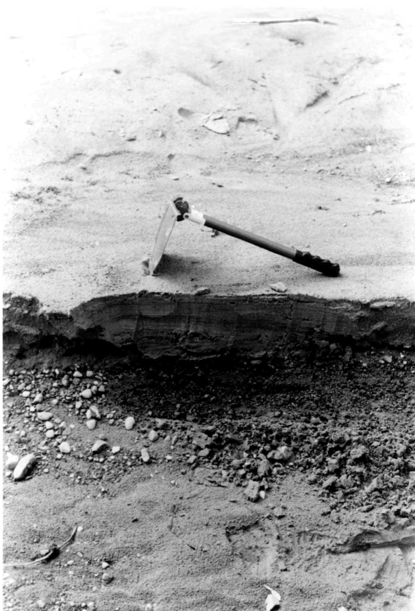
FIGURE 17. Horizontal lamination on the surface of the point bar at C-C - distal sections. The laminae that are illustrated in the photograph are representative of the sediment facies shown in the lower left of Figure (16). The substratum of gravel is significantly finer than the surface lag of the proximal and middle sections of the point bar. The material is coarse sand to fine gravel in size. The view is from right to left.
