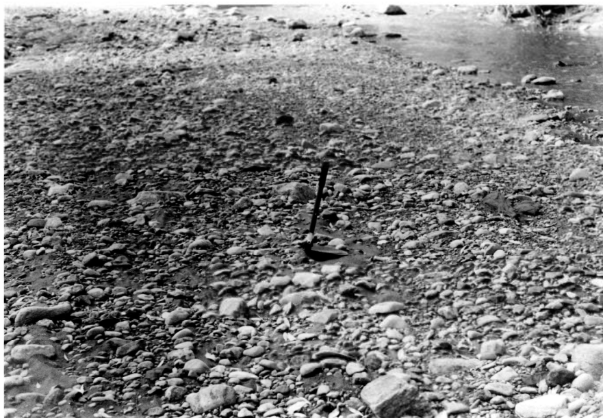
FIGURE 15. The riffle bar surface at E-E. The photograph illustrates the armoured surface of the riffle bar at the proximal end of the feature. The gravel clasts consist of elongate/prolate cobbles and imbricated discoidal clasts, and larger occurrences of clasts that range from rhombohedral to spherical in shape. The flow is towards the reader.
